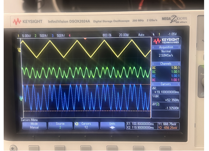
FIG. 12. Shows the signals for the MZ when in scan mode. The yellow represents the ramp signal produced by the PZT moving the mirrors back and forth allowing us to perform a cavity scan. The green is the transmission signal from the MZ's photodiode, and the blue is the accompanying error signal.
