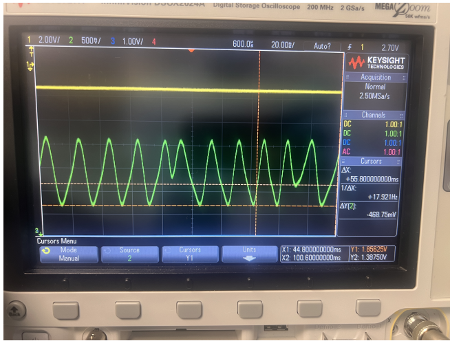
FIG. 14. The OPA signal showing the amplification and deamplification of the beam. The dashed line in the middle of the signal represents no amplification (meaning no green light being sent into the OPA) and acts as our zero line.
