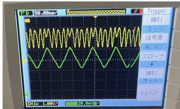
Figure 6: Oscillations in the Fringes of the Michelson Interferometer (Yellow) given an Amplified Periodic Triangular Signal from Function Generator (Green)
