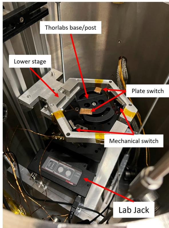
Figure 3: Vacuum system lower stage
