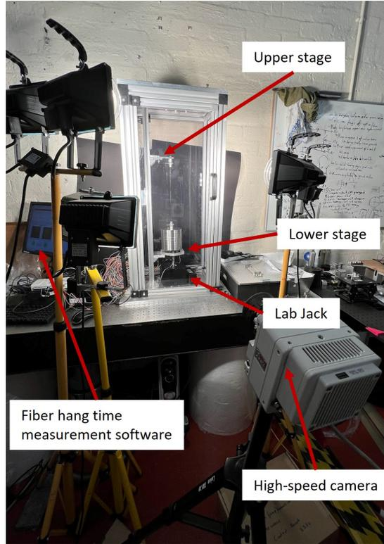
Figure 2: Fused silica fiber lifetime experimental setup
