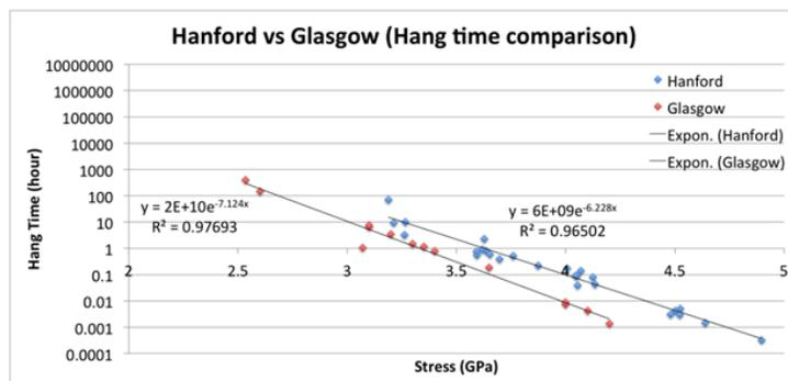
Figure 1: Fiber lifetimes under varying stress. Note that the offset of data sets comes from a difference in the fiber profilers at the two sites.
