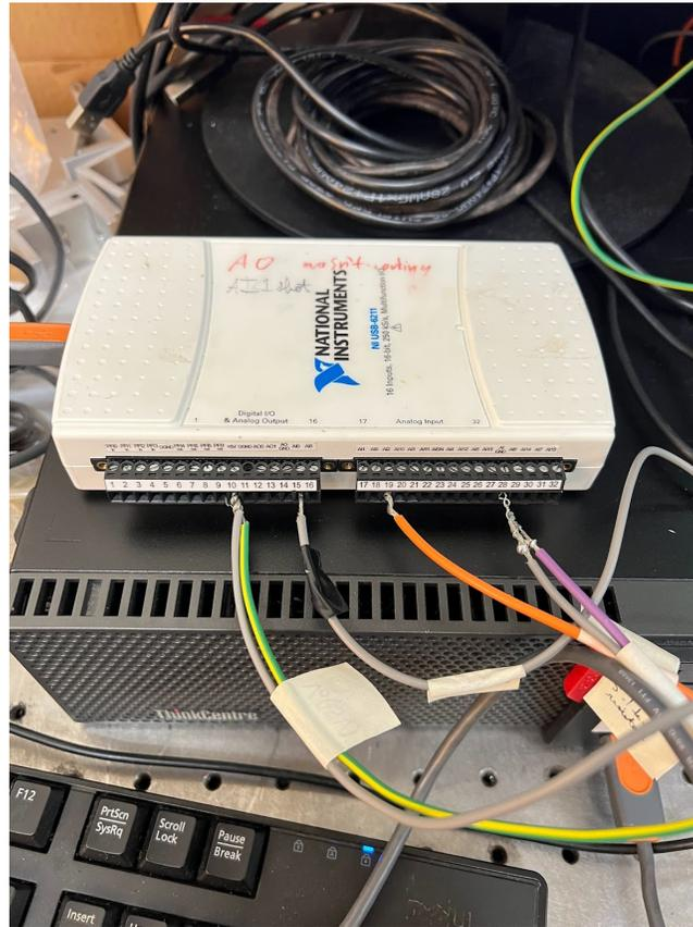
Figure 7: National Instruments analog-digital converter
