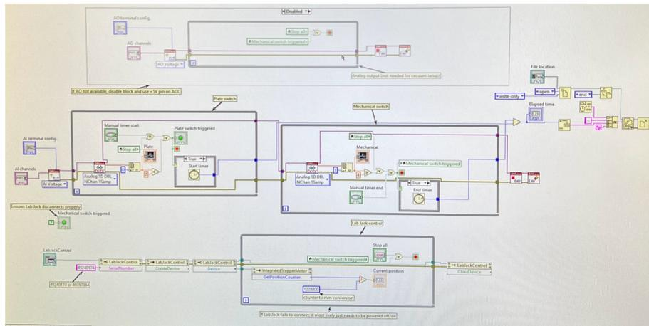
Figure 4: LabVIEW voltage measurement block diagram
