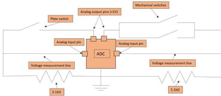
Figure 5: Timing measurement circuit
