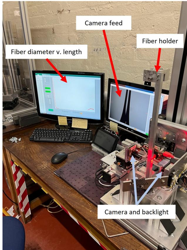
Figure 6: Fiber profiling setup
