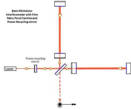
FIG. 1. a basic Michelson interferometer
