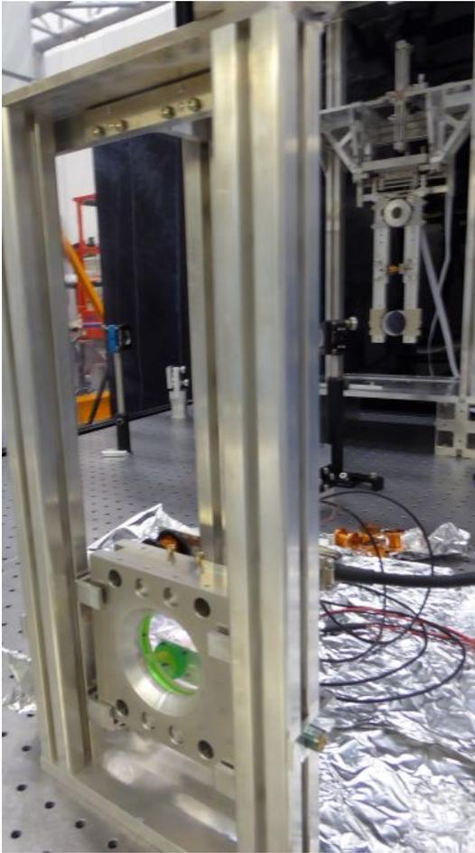
FIG. 12. Close up of mirror in suspension system
