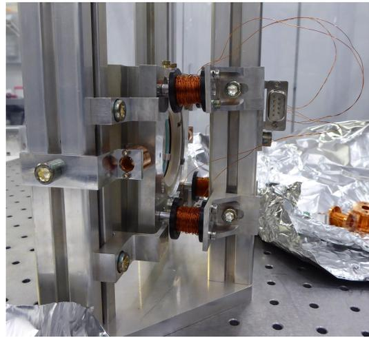
FIG. 10. The suspension system with copper coil damping system
