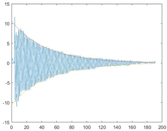
FIG. 20. the amplitude of the signal from the eddy current damping case
