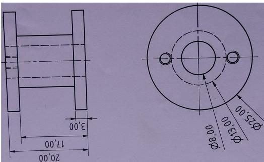
FIG. 6. Design and dimensions of coil holders for suspension system
