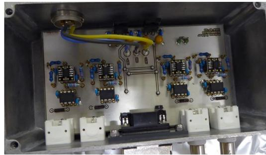
FIG. 11. Negative impedance converter circuit box
