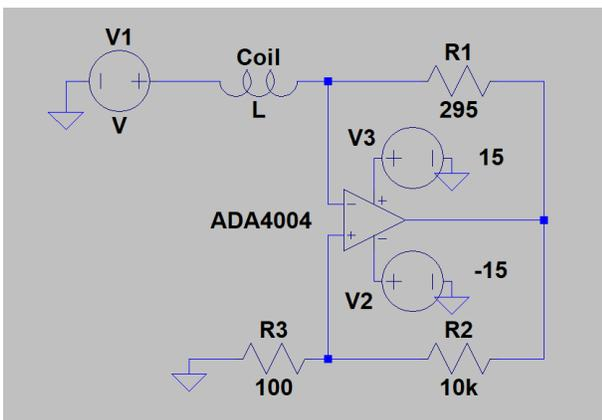
FIG. 4. Negative Impedance Circuit designed on LT SPICE
