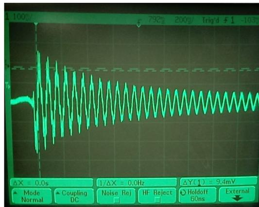
FIG. 5. Signal from oscillating magnet on a wire
