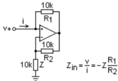
FIG. 3. Negative Impedance Converter from THE Art of Electronics
