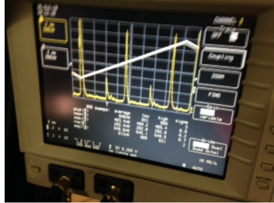
FIG. 6: An oscilloscope reading which shows modes at certain frequencies are resonating inside the cavity. The large peak represents the fundamental mode while the shorter peaks represent the higher order modes that are also resonating. Taking the area under the curve of all the peaks will tell us about the percentage of power that is going to each resonating mode. In a perfect setup, the fundamental mode is the only mode that should be resonating.
