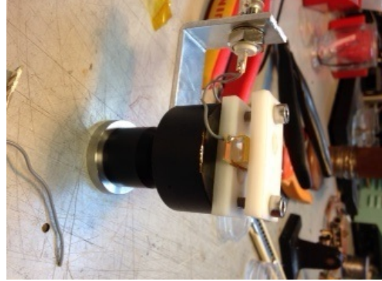
FIG. 9: An EOL sandwiched between two specially-designed copper electrode plates with wire attached to a connector to apply a voltage.
