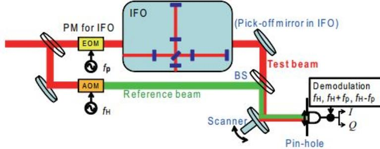
Figure 1: Phase camera set-up.
