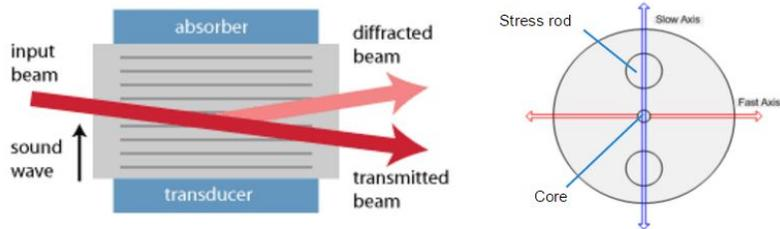
Figure 2: AOM operation mechanism and polarization maintaining fiber.
