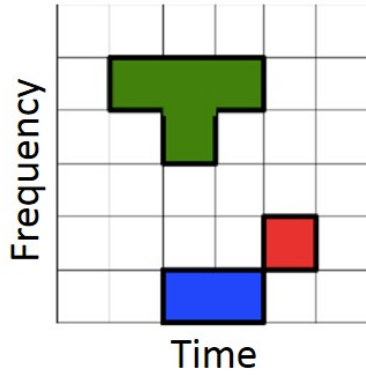
Figure 1: A time frequency map with pixels grouped into 3 clusters, denoted by different clusters. Each cluster is considered a candidate signal event.
