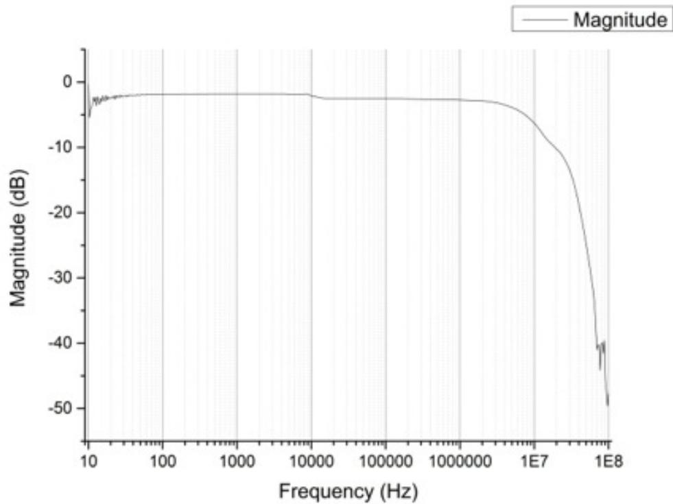
**Fig. 5 Typical transfer function curve for current buffer.**
