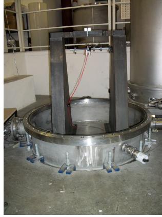
Figure 2.1: Steel structure used to suspend the fiber
