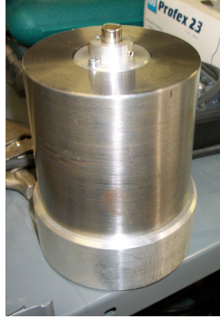
Figure 2.4: The 5 kg mass with the magnet attached
