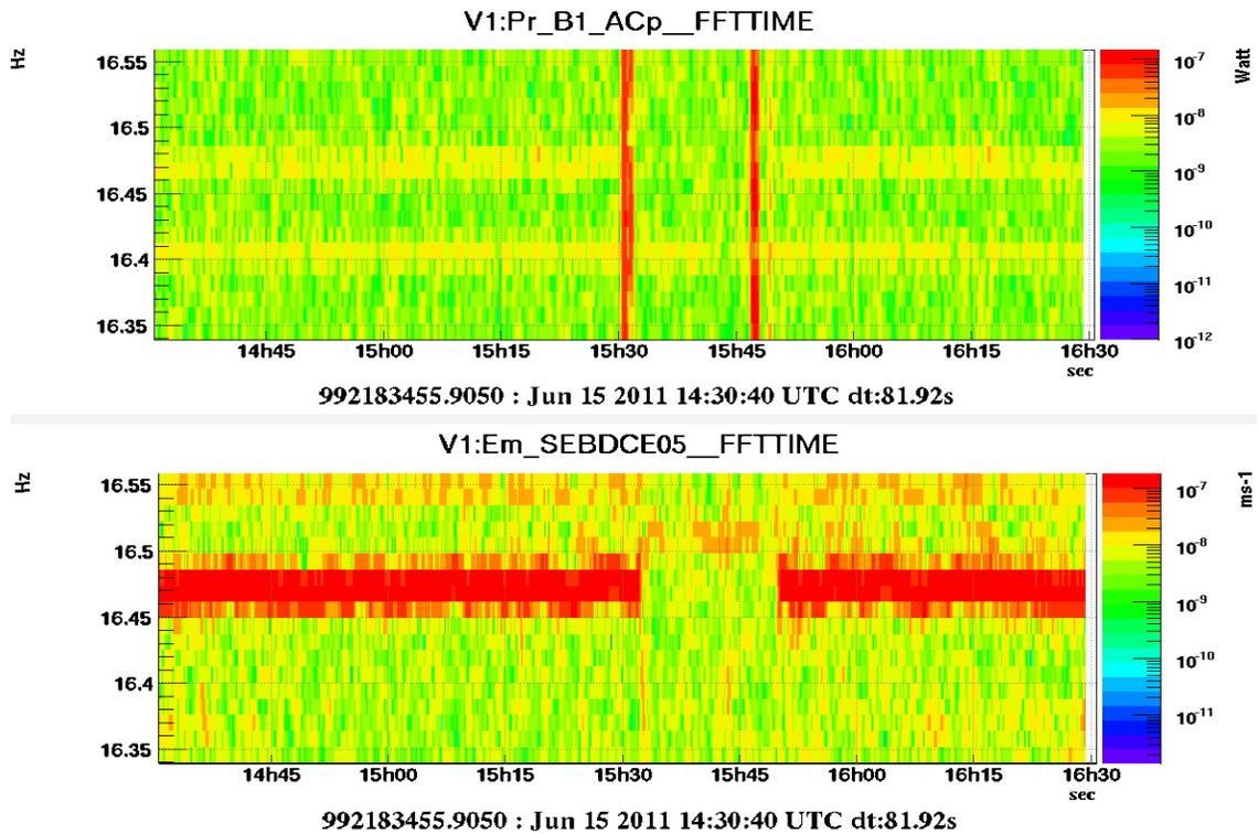
FIG. 9: A spectrogram (frequency vs. time) of the dark fringe (V1:Pr\_B1\_ACp) and a seismometer (V1:Em\_SEBDCE05) in the central building during the shut off test reveals that the source of the noise line at 16.46 Hz is the air conditioner in the injection clean room located in the central building.
