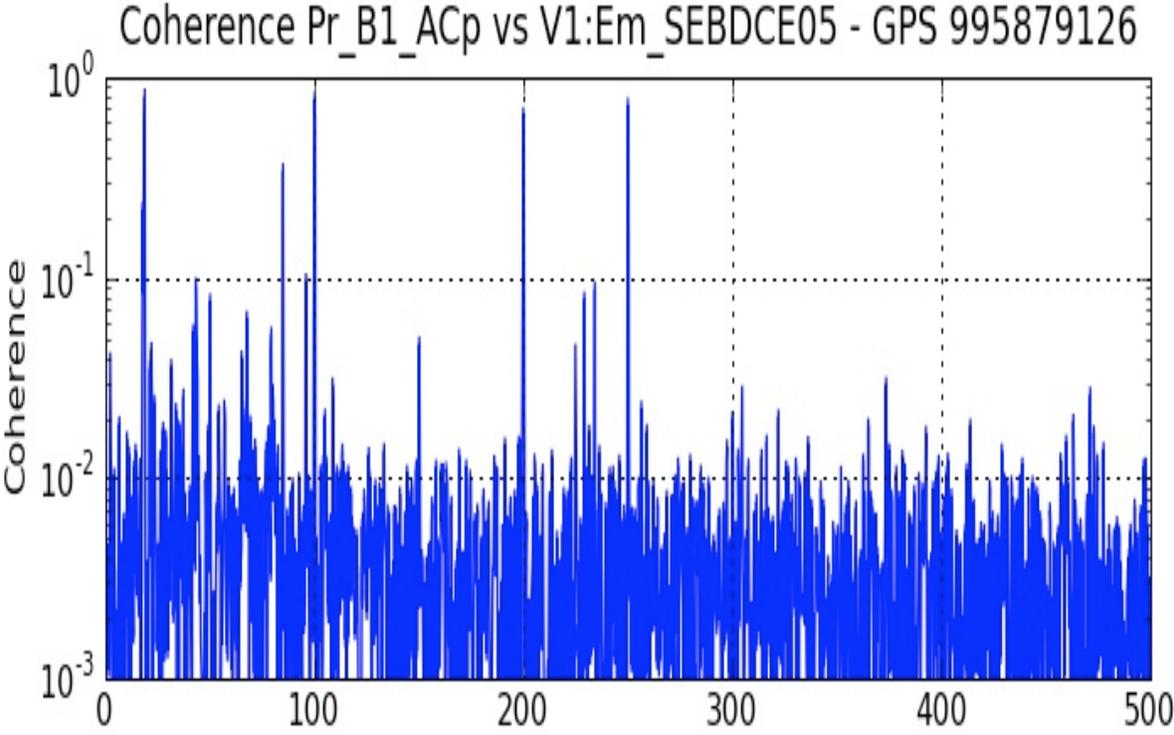
FIG. 3: A plot (coherence vs. frequency) showing the amount of coherence between the dark fringe (Pr\_B1\_ACp) and a seismometer (V1:Em\_SEBDCE05) located in the central building between 0 and 500 Hz on July 28, 2011. High coherence is visible at frequencies of 20, 100, 200, and 250 Hz.
