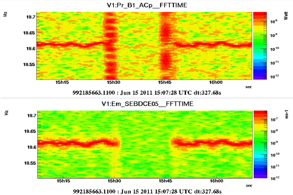
FIG. 12: A spectrogram (frequency vs. time) of the dark fringe (V1:Pr\_B1\_ACp) and a seismometer (V1:Em\_SEBDCE05) in the central building during the shut off test reveals that the source of the noise line at 18.61 Hz is the fan in the detection lab located in the central building.
