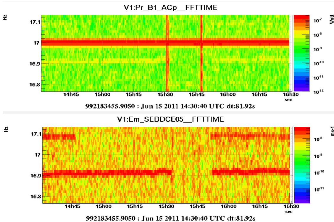
FIG. 10: A spectrogram (frequency vs. time) of the dark fringe (V1:Pr\_B1\_ACp) and a seismometer (V1:Em\_SEBDCE05) in the central building during the shut off test reveals that the source of the noise line at 16.9 Hz is the air conditioner in the data acquisition room located in the central building.
