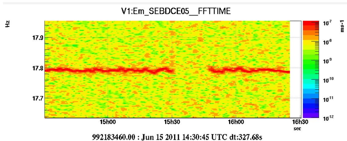
FIG. 11: A spectrogram (frequency vs. time) of a seismometer (V1:Em\_SEBDCE05) in the central building during the shut off test reveals that the source of the noise line at 17.78 Hz is the fan in the detection lab located in the central building.
