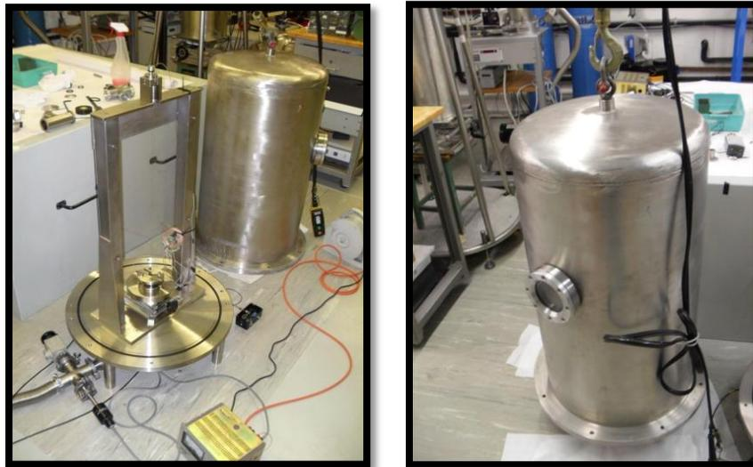
*Figure 1: mounting mechanism designed to support fiber (left) and the chamber (right) used to create a suitable vacuum to simulate Virgo conditions*
