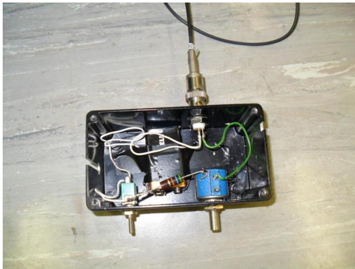
*Figure 6. LED lighting system control box*
