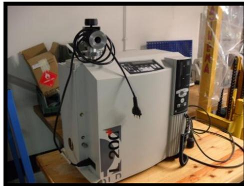
**Figure 5:** Image of leak detector.
