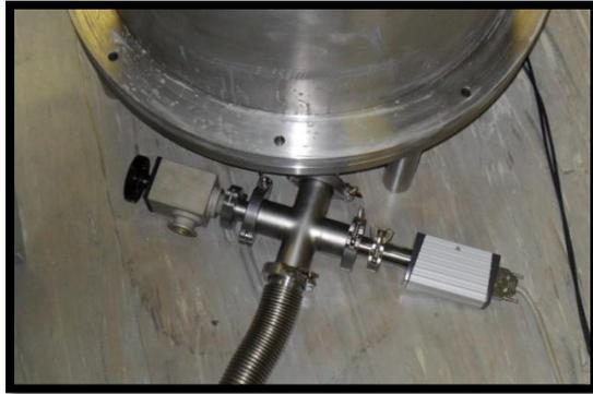
**Figure 4:** Picture of pipe set up with air inlet (left) and Vacuum gauge sensor (right) attached.
