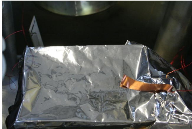
Figure 4: Image of heater box used in specially designed vacuum chamber
